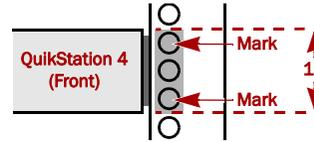
Use these holes if the rack length  $\geq$  unit length
